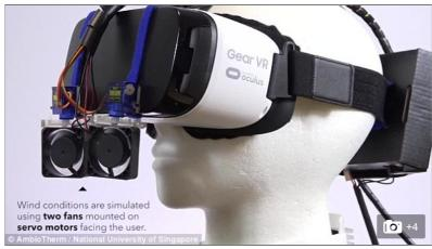
The thermal stimulation module is attached to the user's neck while two fans on the user's face simulate wind conditions
